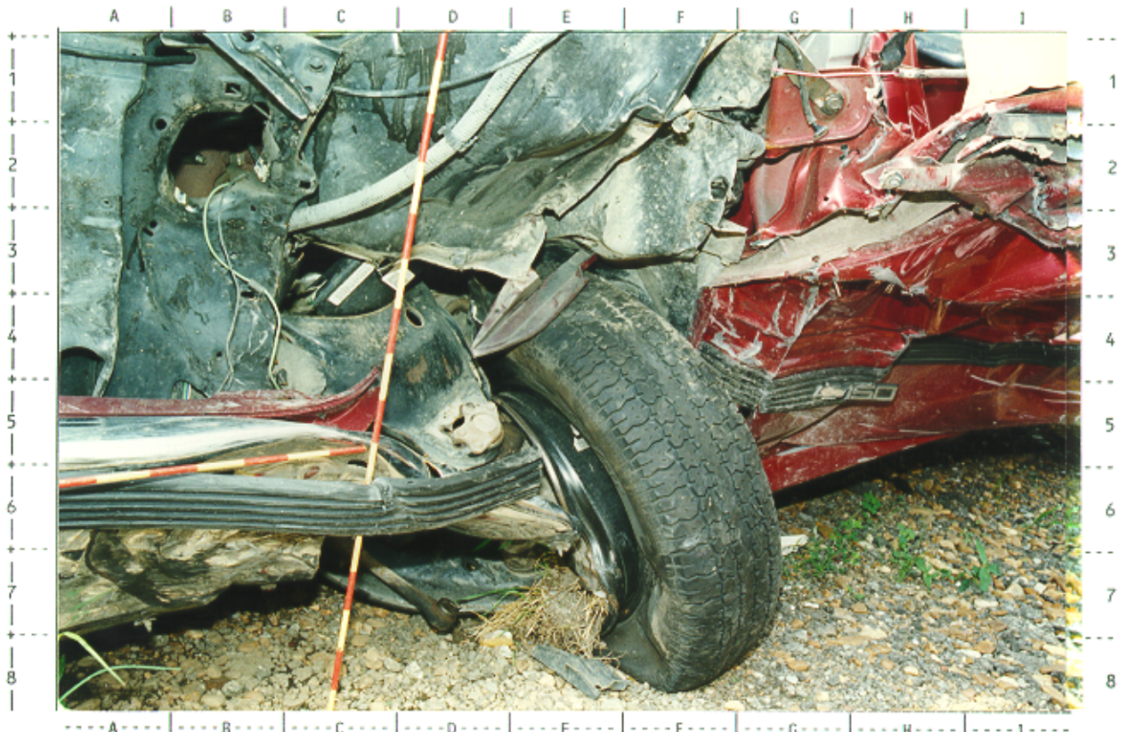
# 68 -- Close-up of 1988 Chevrolet pickup's left front wheel damage; NOTE: broken steering rod and grass & mud in wheel rim
